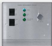
► GREASE MASTER energy management systems (EMS) reduce exhaust and supply airflow rates, saving restaurant operators energy and money. A digital temperature control modulates fans between fully adjustable high and low speeds to meet your exact exhaust requirements. The energy management system saves energy in three places – fan energy, make-up air, and transfer air. The EMS package also meets IMC 507.2.1.1.
